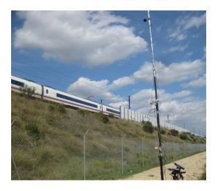
Tasks being developed by AV Ingenieros in collaboration with Russian researchers will allow validating a prediction model of noise induced by high-speed railway lines.
